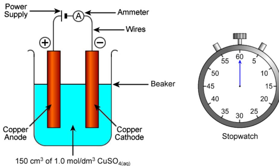
**Note:** It is possible to use a graphite cathode for this experiment, but a copper anode should be used to ensure that the concentration of copper(II) ions in solution remains constant.
