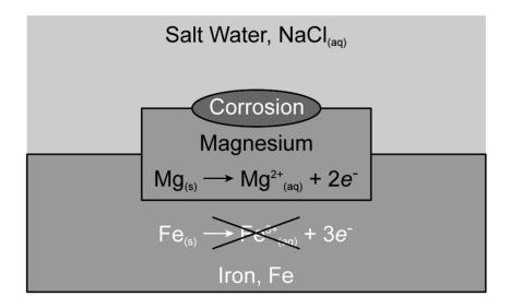
Describe how sacrificial protection prevents the iron from corroding / rusting.
