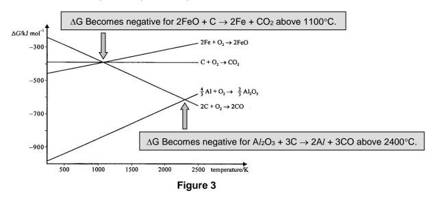
Whereas reduction of iron(II) oxide by carbon is feasible ( $-\Delta G$ ) at about 1100°C, reduction of aluminium oxide by carbon is only feasible ( $-\Delta G$ ) at about 2400°C. To reach such a high temperature requires a huge amount of energy and is therefore not financially viable.
