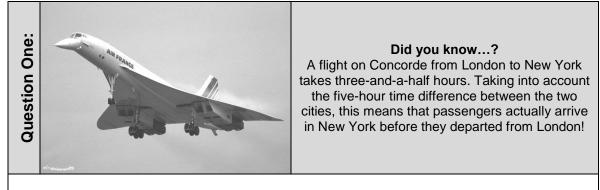
Concorde was the World's only supersonic passenger airliner. When flying over the Atlantic ocean at a height of 17.7 km and a speed of 2170 km / h (twice the speed of sound), Concorde's external airframe reached a temperature of 130°C at the nosecone and 90°C at the tail. This caused Concorde to expand in length from 62.10 m to 62.22 m.
